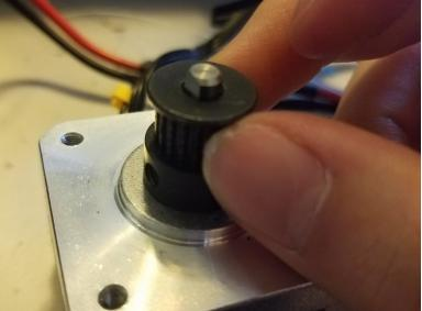
Loosen this grub screw on the stepper just enough so that the gear can be smoothly moved up and down by hand. There may be a second grub screw set at about 90 degrees from the first one, loosen that one too
