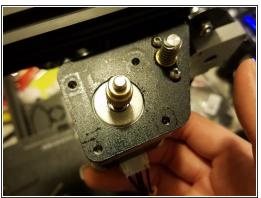
Note: The Extruder motor is held up by three screws and nothing else: Removing these screws will cause your motor to fall to the table
