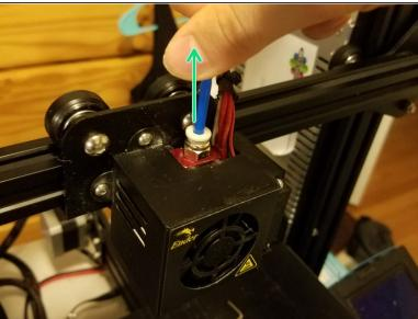
Safety note: While doing this, hold onto the fan housing and not the gantry arm to avoid burning yourself
