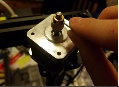
With the motor out, loosen the two grub screws holding the drive gear in place, and remove it.
