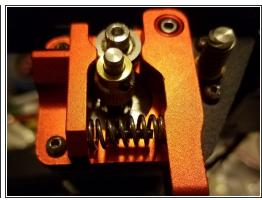
Place one of the hex screws you removed from the stock motor frame inside of the new spring, then compress it and slide it into position between the idler arm and frame.
