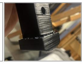
Insert the inner box into the outer box so it fits snugly, and fit the foot into the bottom of the inner leg.
