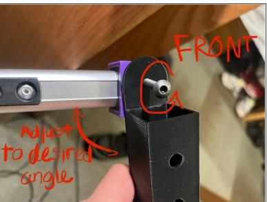
Adjust the angle as needed until the desired height above the ground is reached. Then, place the nut on the outer box hole on the side closer to the center of the wheelchair and place the screw through the hole in the nut. Finally, tighten the nut until the outer leg is securely in place.
